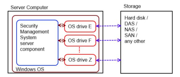
This provides full flexibility in system design and allows using any type of storage with Security Management System. As long as the storage is able to reflect one or more 'drives' in Windows OS, Security Management System is able to access it and use it for data storage.
